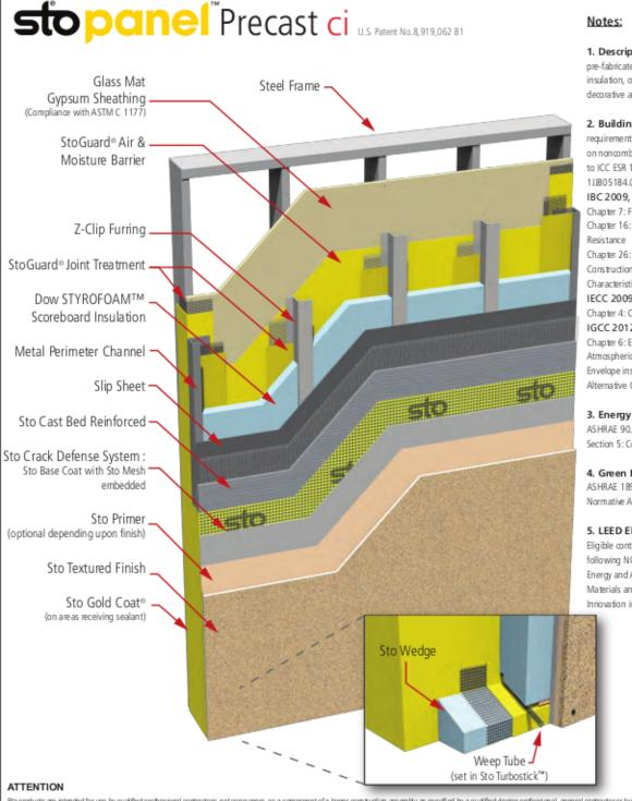
1. Description: lightweight energy efficient pre-fabricated exterior wall panel with exterior insulation, continuous air barrier, and integral decorative and protective finish options
